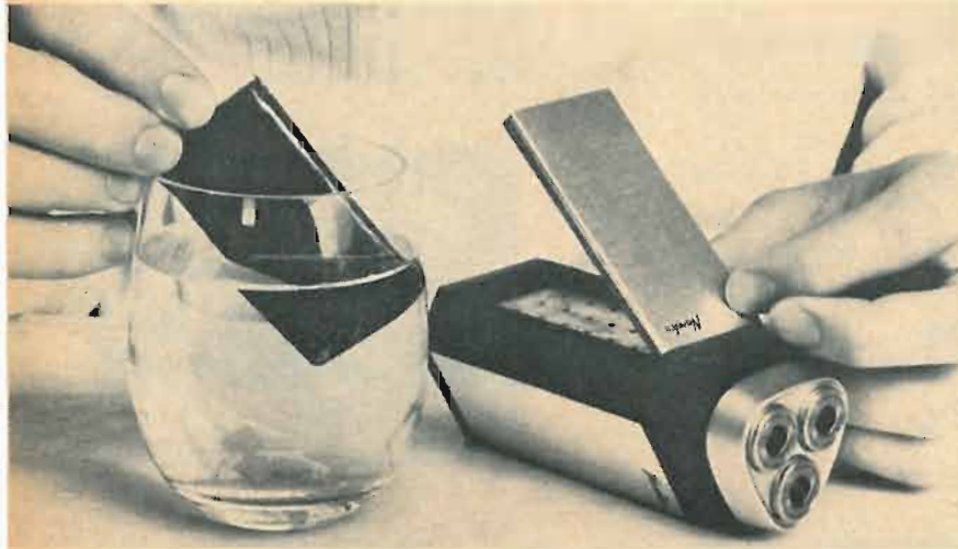
Disposable power cell is moistened before use, activating chemically treated fibers. Metallic plate on the shaver's lid serves as top layer in cell "sandwich" and must be replaced periodically. Top layer is equivalent to zinc can in conventional cell.
